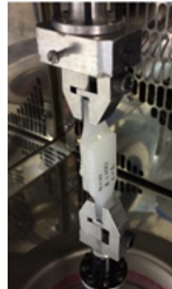
FIGURE 5. Specimens bonded by the adopted ultrasonic joining device.
