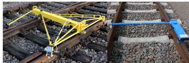
FIGURE 3. Trolley Krab (track geometry) [5] and Salamander (corrugations)
