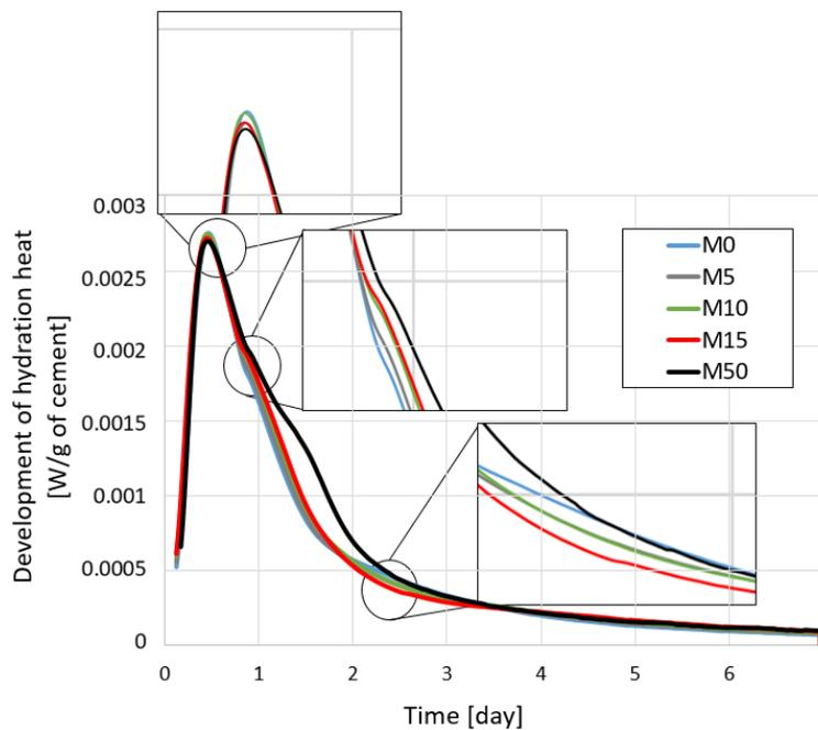
FIGURE 2. Curve of heat evolution for tested materials.
