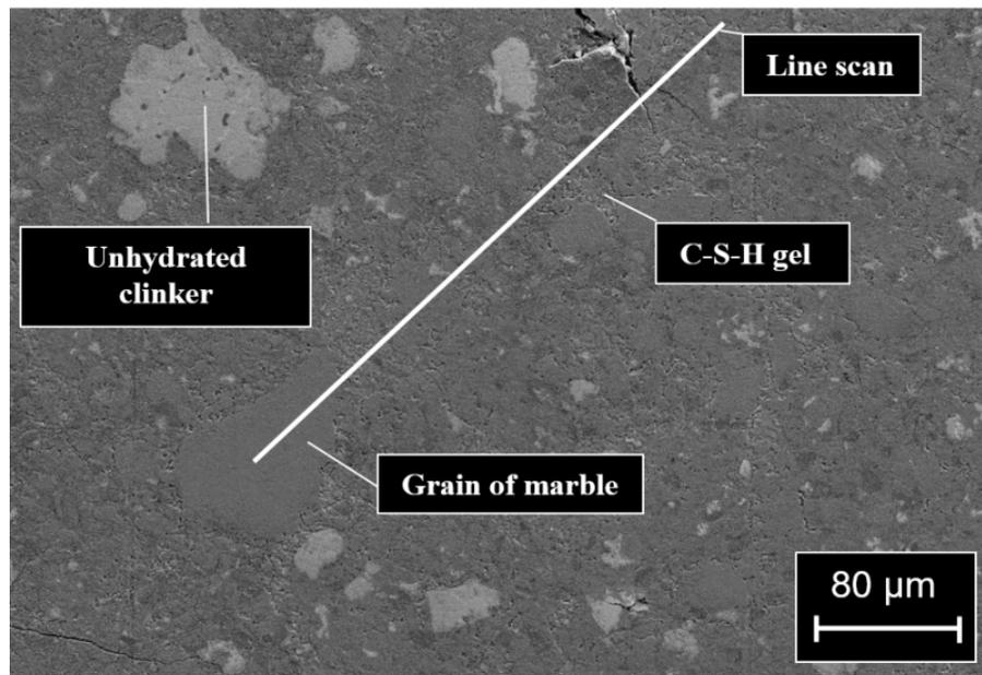
FIGURE 3. The image of cement paste containing micronized marble powder, magnified 500×.
