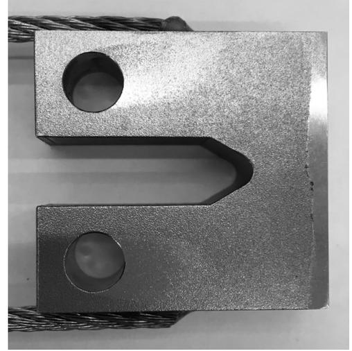
FIGURE 4. The blunt notch CT specimen used in the current study; image from Ref. [6].
