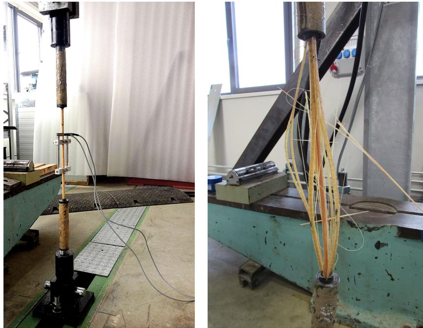
FIGURE 4. Cyclic test configuration with LVDTs (left), broom-like failure mode with an undamaged core (right).
