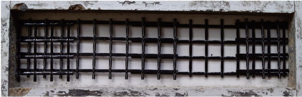
FIGURE 1. View in the wooden mold just before casting process on the used flat carbon concrete reinforcement with overlapping in the middle part.
