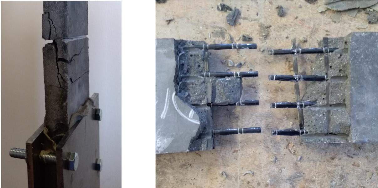
FIGURE 4. Typical detailed pictures of damaged specimens with shear collapse during testing procedure and just after the collapse of specimens and its uninstalling from the testing machine.
