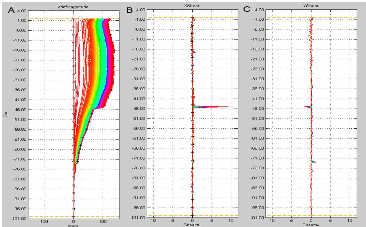
FIGURE 10. Magnitude of displac. (A), X shear stress (B), Y shear stress (C), Belchatow mine.
