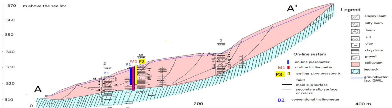
FIGURE 2. Geological engineering cross-section of landslide in Szymbark.
