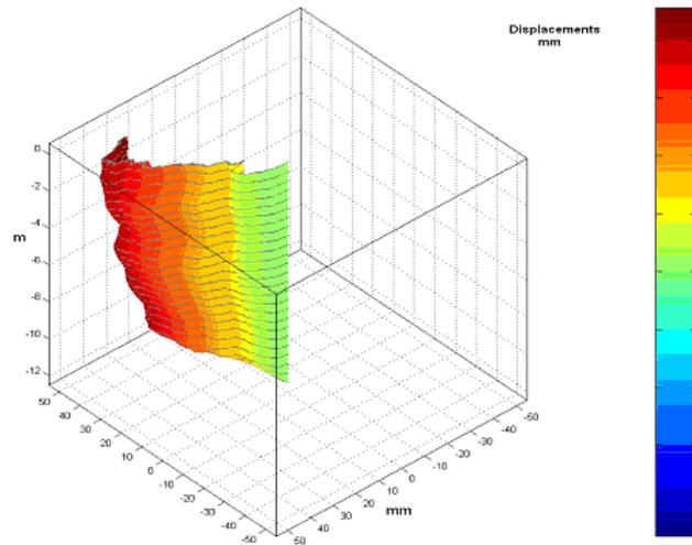
FIGURE 6. Ground displacement 3D model, Szymabark landslide.
