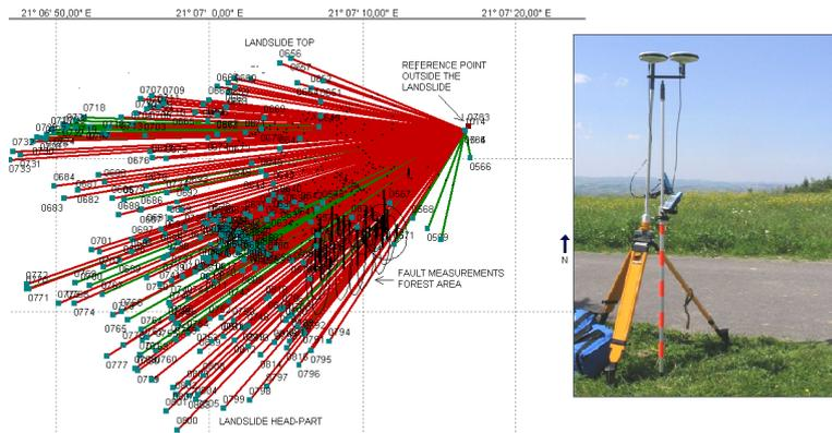
FIGURE 4. GPS-postprocessing results, Szymbark landslide.
