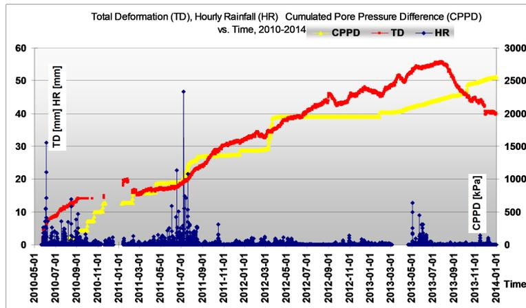
FIGURE 7. Results of on-line displacement, rainfall and pore pressure measurements, Szymabark.
