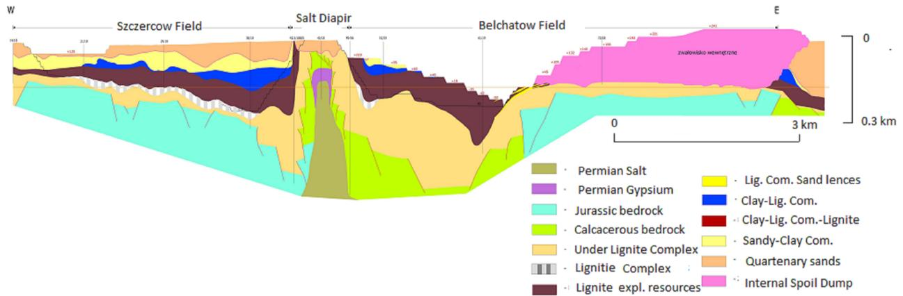
FIGURE 9. Geological WE cross-section of Belchatow and Szczercow Fields.
