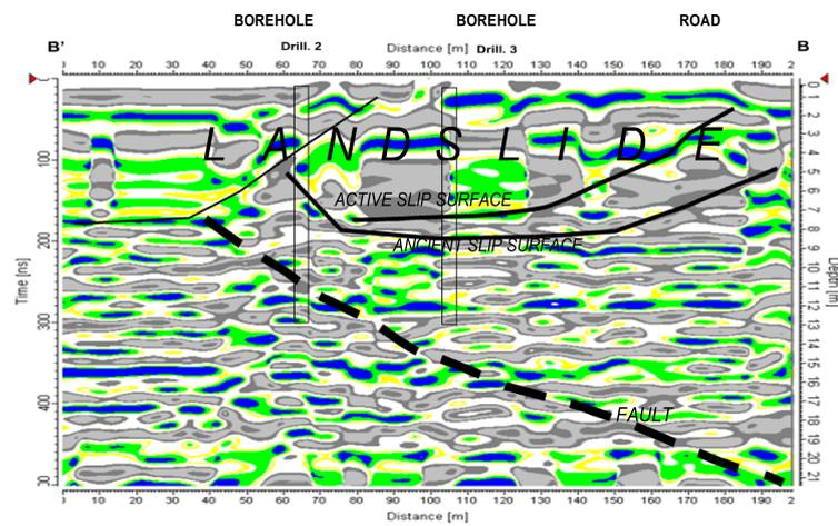
FIGURE 3. Sekowa landslide GPR scanning results.
