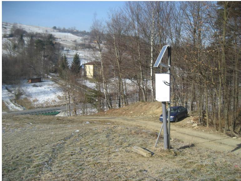
FIGURE 5. Online landslide monitoring station, Szymbark landslide.
