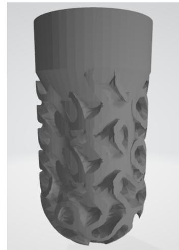
FIGURE 3. The second, porous geometrical solution of the dental implant used for numerical simulations. Implant was previously patented in the Czech Republic [7]. Image shows the intraosseous part.
