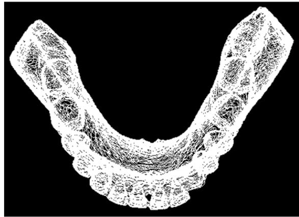
FIGURE 5. The wireframe model of the human mandible for the creation of the FEM mesh. The left canine was extracted in the step of ROI extraction as dental implants will be introduced.
