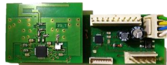
Fig. 6. ZigBee network router & coordinator all in one node.
