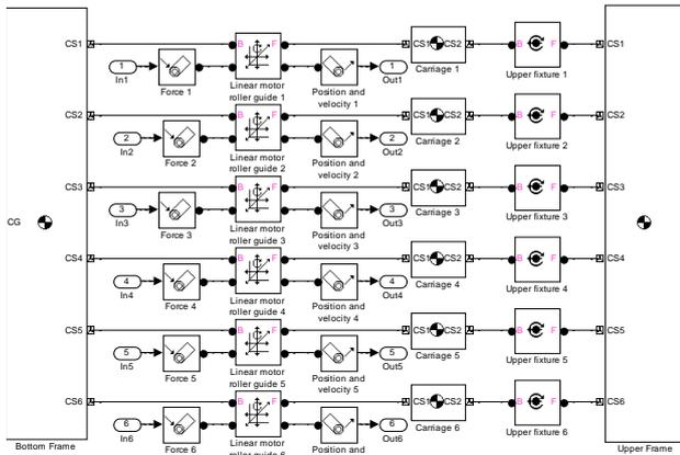
Fig. 3: Mathematical Model of the Mechanism in the MATLAB/Simulink/SimMechanics Environment.
