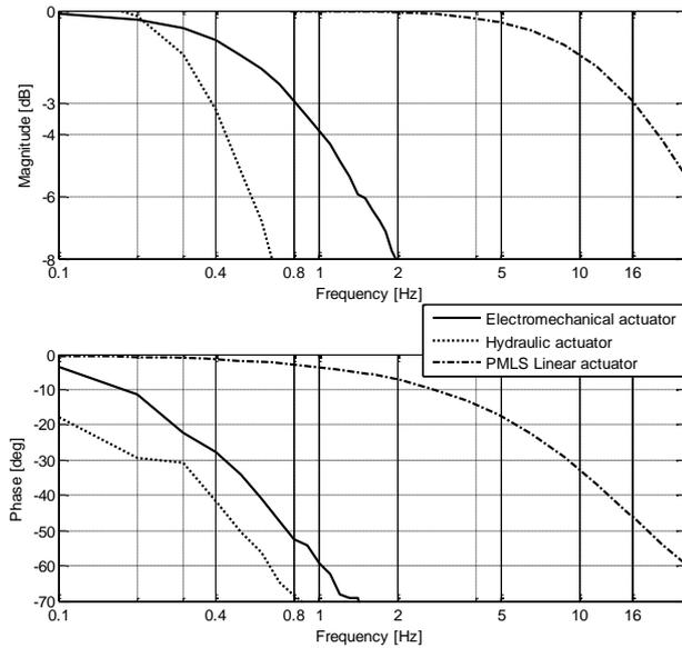
Fig. 5: Frequency characteristics
