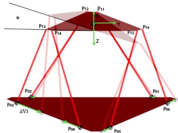
Fig. 1: Motion Platform with Six Degrees of Freedom Driven by Linear Actuators
