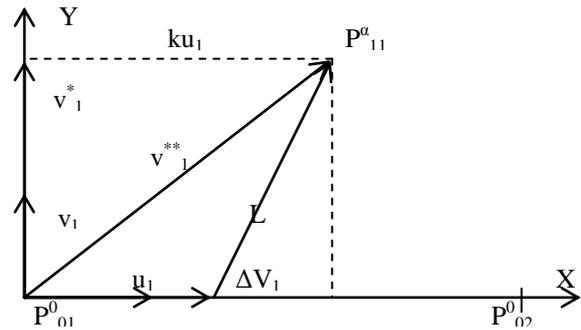
Fig. 2: Vector analysis of the linear motor displacement calculation
