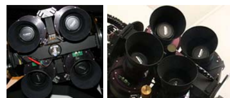
Fig. 5: Two modes: side-by-side (left) and common target (right)
