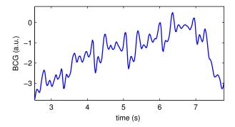
FIGURE 7. Band-pass filtered BCG data  $(0.5-20\,\mathrm{Hz})$  with respiratory influence.
