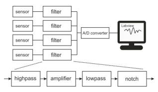
FIGURE 2. Analog filter chain.
