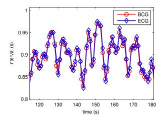
FIGURE 11. Comparison of BCG and ECG beat-to-beat interval estimation.
