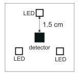
FIGURE 3. Sensor PCB.
