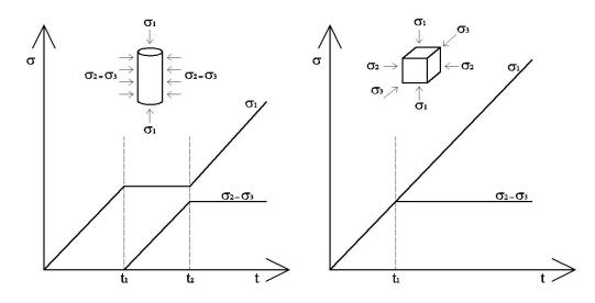
FIGURE 1. Testing procedure for UHPC cylinders and cubes.
