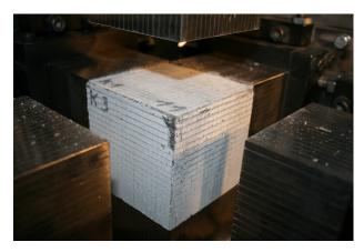
FIGURE 2. Triaxial hydraulic loading machine.
