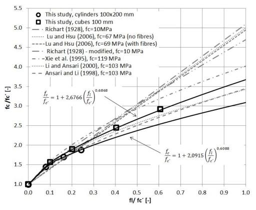
FIGURE 3. Development of triaxial compressive strength.
