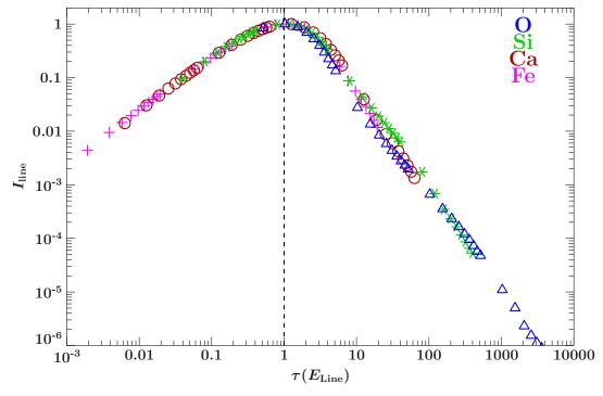
Figure 5. General line shape for a spherical geometry and for a monochromatic photon beam at  $E=10\,\mathrm{keV}$  as input.
