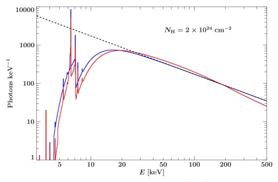
FIGURE 1. Absorbed spectra transmitted through a sphere for  $N_{\rm H} = 2 \times 10^{24} \, {\rm cm}^{-2}$ . The red spectrum is calculated with considering Compton scattering, the blue one with including photo absorption only. The dashed line indicates the input spectrum.
