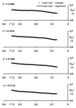
FIGURE 8. Dimensionless axial mean velocity profile  $\overline{u_r}/(ND) = f(r^*)$ .
