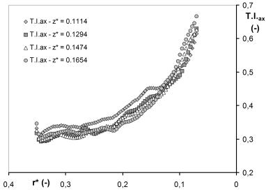
FIGURE 10. Axial turbulence intensity profile  $\mathrm{TI}_{\mathrm{ax}} = f(r^*)$ .
