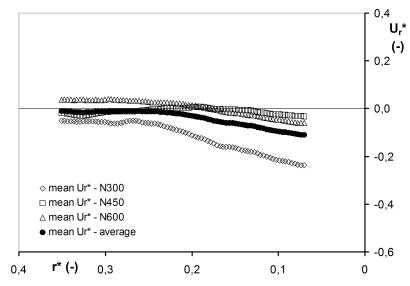
Figure 2. Dimensionless radial mean velocity profile – effect of impeller speed;  $z^* = 0.1474$ .
