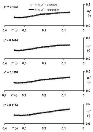
FIGURE 7. Dimensionless radial fluctuation velocity profile  $\overline{U_{\rm ax}}/(ND)=f(r^*)$ .
