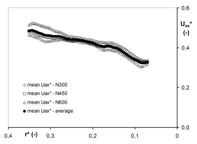
FIGURE 4. Dimensionless axial mean velocity profile – effect of impeller speed;  $z^* = 0.1474$ .
