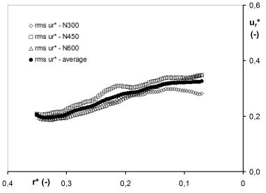
Figure 3. Dimensionless radial fluctuation velocity profile – effect of impeller speed;  $z^* = 0.1474$ .
