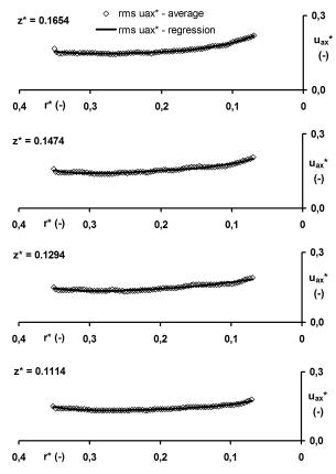
FIGURE 9. Dimensionless axial fluctuation velocity profile  $\overline{u_{\rm ax}}/(ND) = f(r^*)$ .
