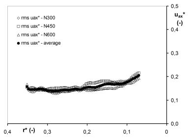
FIGURE 5. Dimensionless axial fluctuation velocity profile – effect of impeller speed;  $z^* = 0.1474$ .
