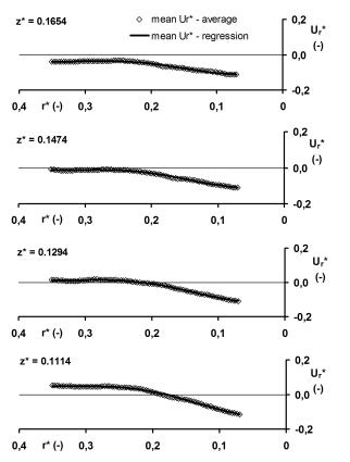
FIGURE 6. Dimensionless radial mean velocity profile  $\overline{U_r}/(ND) = f(r^*)$ .
