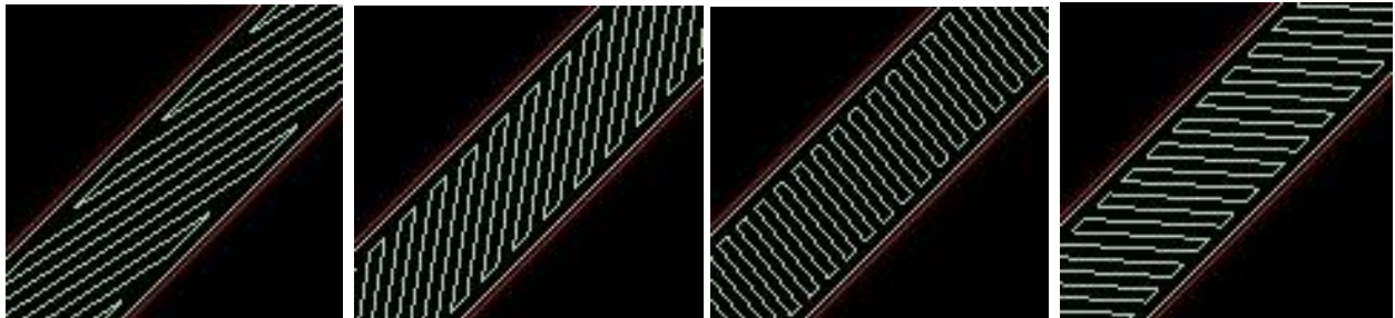
FIGURE 7. Direction of the fibers on different layers of PC specimens – 45 degrees.
