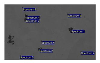
FIGURE 6. Analysed zones of microstructure in Bi2La solder.
