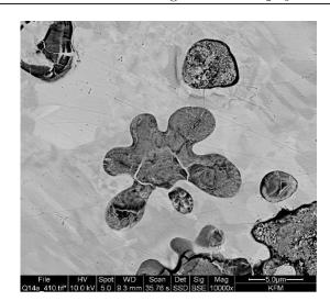
FIGURE 5. Microstructure of Bi2La solder with La phases and microstructure with twins.
