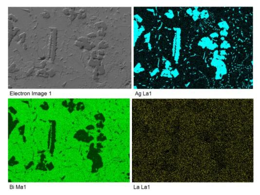
FIGURE 4. Planar analysis of BillAg2La solder.
