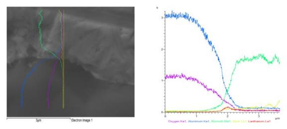
FIGURE 8. Concentration profiles of Bi, La, Ag, Al and O elements on the boundary of Al<sub>2</sub>O<sub>3</sub>/Bil1Ag2La joint.
