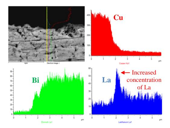
FIGURE 7. The EDX analysis of Cu/Bi2La joint boundary with concentration of Bi, La and Cu elements.
