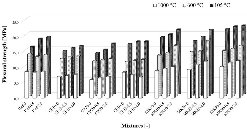
FIGURE 2. Flexural strength of the tested composites.
