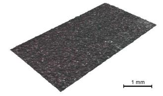
FIGURE 8. Non-filtered image of the surface of sample 30,  $2.5 \times$  magnified (voltage 70 V,  $T_{\rm on}=6\,\mu \rm s$ ,  $T_{\rm off}=30\,\mu \rm s$ , wire feed  $14\,\rm m/min$ , current  $35\,\rm A$ ).
