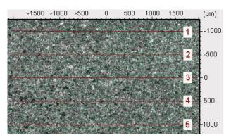
FIGURE 3. Position of distribution of areas for waviness measurement.
