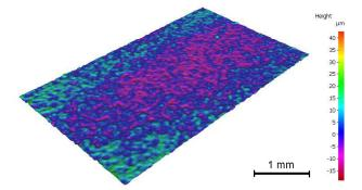
FIGURE 5. Colour filtered image of the surface of sample 23,  $2.5 \times$  magnified (voltage 70 V,  $T_{\rm on}=10\,\mu s$ ,  $T_{\rm off}=30\,\mu s$ , wire feed 14 m/min, current 25 A).
