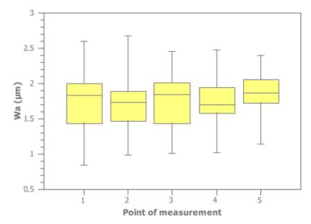
FIGURE 9. Values Wa in individual points of measurement on all samples made of titanium alloy Ti-6Al-4V.
