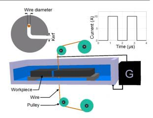
FIGURE 1. Diagram of wire electrical discharge machining process.
