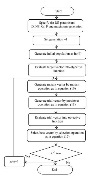
FIGURE 2. Flowchart of differential evolution.
