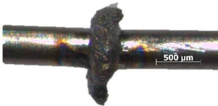
FIGURE 16. RBW sample 0.46 mm, etched wire.
