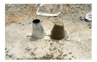
FIGURE 4. Slump with EPS bead at  $12.5\,\%$  replacement.
