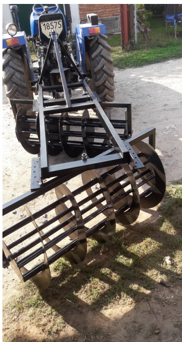
FIGURE 9. Overall view of the harrow equipped with helical tools.
