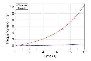
FIGURE 6. A frequency error between a logarithmic chirp signal generated by 24-bit fixed-point arithmetic with different coercing options, truncate and round and a floating-point generation. Signal parameters  $f_s = 10 \ kHz$ ,  $f_{start} = 10 \ Hz$ ,  $f_{stop} = 100 \ Hz$ .
