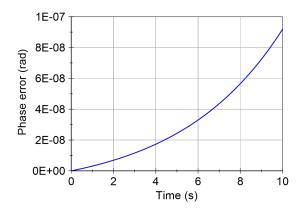
FIGURE 3. A phase error between the logarithmic chirp signal generated by a numerical integration using the trapezoidal rule and a LabVIEW built-in function. Signal parameters  $f_s = 10 \ kHz$ ,  $f_{start} = 10 \ Hz$ ,  $f_{stop} = 100 \ Hz$ .
