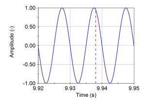
FIGURE 9. Detail of the transition between the chirp and sine signal generated by our 32-bit fixed-point generator.
