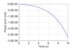
FIGURE 4. A phase error between logarithmic chirp signal generated by an analytical integration using fixed-point and floating point representation. Signal parameters  $f_s = 10 \ kHz$ ,  $f_{start} = 10 \ Hz$ ,  $f_{stop} = 100 \ Hz$ .
