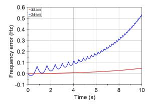
FIGURE 5. A frequency error between a logarithmic chirp signal generated by 24 and 32-bit fixed-point arithmetic with rounding and a floating-point generation. Signal parameters  $f_s = 10 \ kHz$ ,  $f_{start} = 10 \ Hz$ ,  $f_{stop} = 100 \ Hz$ .
