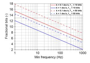
FIGURE 7. A minimal length of a fractional part of a fixed-point number in dependence on a minimal frequency in a chirp signal for different chirp speeds and sampling frequencies.
