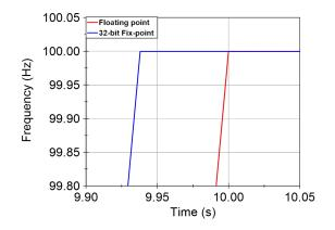
FIGURE 8. Comparison of the actual chirp speed frequency generated on 32-bit fixed-point and floating point arithmetics.
