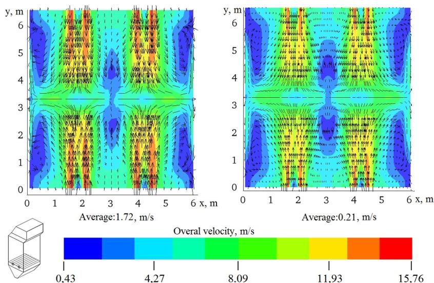
FIGURE 2. The field of the overall velocity vector in the area of the arrangement of the burners for various percentages of air supplied through the injectors: a) OFA = 0 % (basic version), b) OFA = 10 %.
