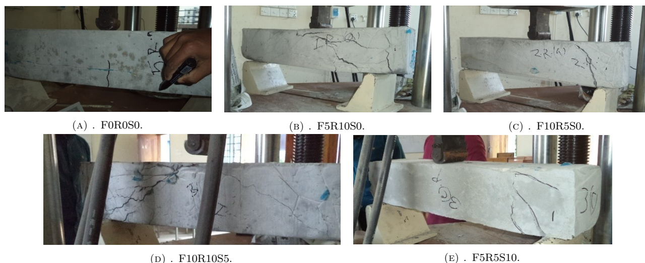
FIGURE 10. Failure mode of RC beam specimens cast with different concrete mixes.
