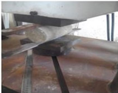
(E) . Splitting tensile strength test.
