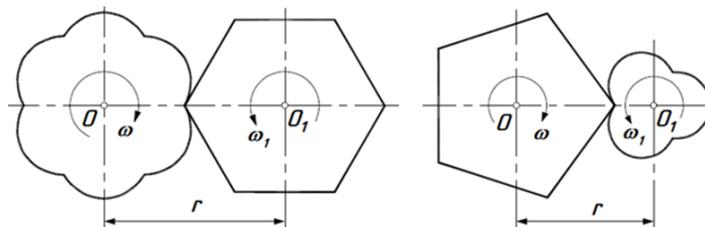
FIGURE 5. Polygons and curvilinear profiles with different numbers of sides and curvilinear elements at  $r = 100$ : a) a hexagon with a radius of the circumscribed circle  $R = 54.93$  and a corresponding curvilinear profile with six elements; b) a pentagon with a radius of the circumscribed circle  $R = 71.47$  and a corresponding curvilinear profile with three elements.
