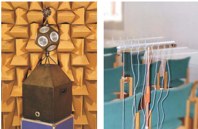
Fig. 2: 3-way dodecahedron loudspeaker (left) and condenser microphones in an array (right)
